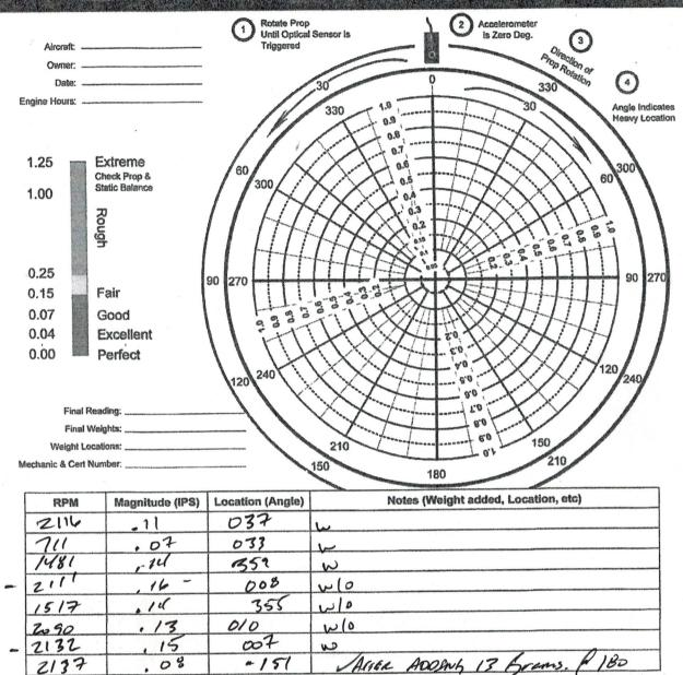
Per AC20-37E: Install a placard on the propeller hub or bulkhead stating that the propeller has been dynamically balanced and the assembly of the power train rotating components is an indexed assembly. Make an entry in the logbook with the date, engine hours, final balance vibration, location of the dynamic balance weights, signature and certificate number of the maintenance person.
