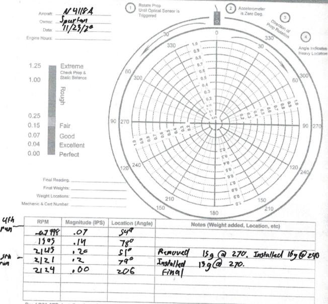
Per AC20-37E: Install a placard on the propeller hub or bulkhead stating that the propeller has been dynamically balanced and the assembly of the power train rotating components is an indexed assembly. Make an entry in the logbook with the date, engine hours, final balance vibration, location of the dynamic balance weights, signature and certificate number of the maintenance person.
