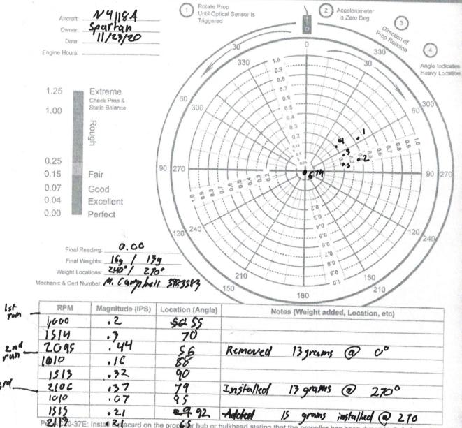
P2AC20-37E: Install Spacard on the propeller hub or bulkhead stating that the propeller has been dynamically balanced and the assembly of the power train rotating components is an indexed assembly. Make an entry in the logbook with the date, engine hours, final balance vibration, location of the dynamic balance weights, signature and certificate number of the maintenance person.
